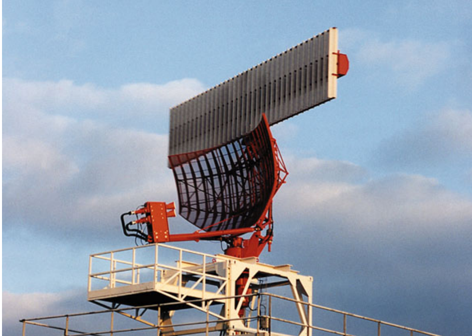
Figure 4: Primary and secondary co-mounted radar antennas
